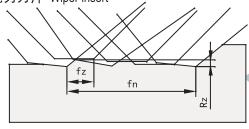
由于刀体和刀片存在制造误差,所以, 刀具存在端刃的端面圆跳动和圆周刃的 径向圆跳动,端刃的端面圆跳动将导致 已加工表面粗糙度Ra值升高,使表面质 量达不到要求。 It has axial and radial run out because of tools and inserts exist manufacturing tolerance. The axial runout lead to poor surface roughness.
